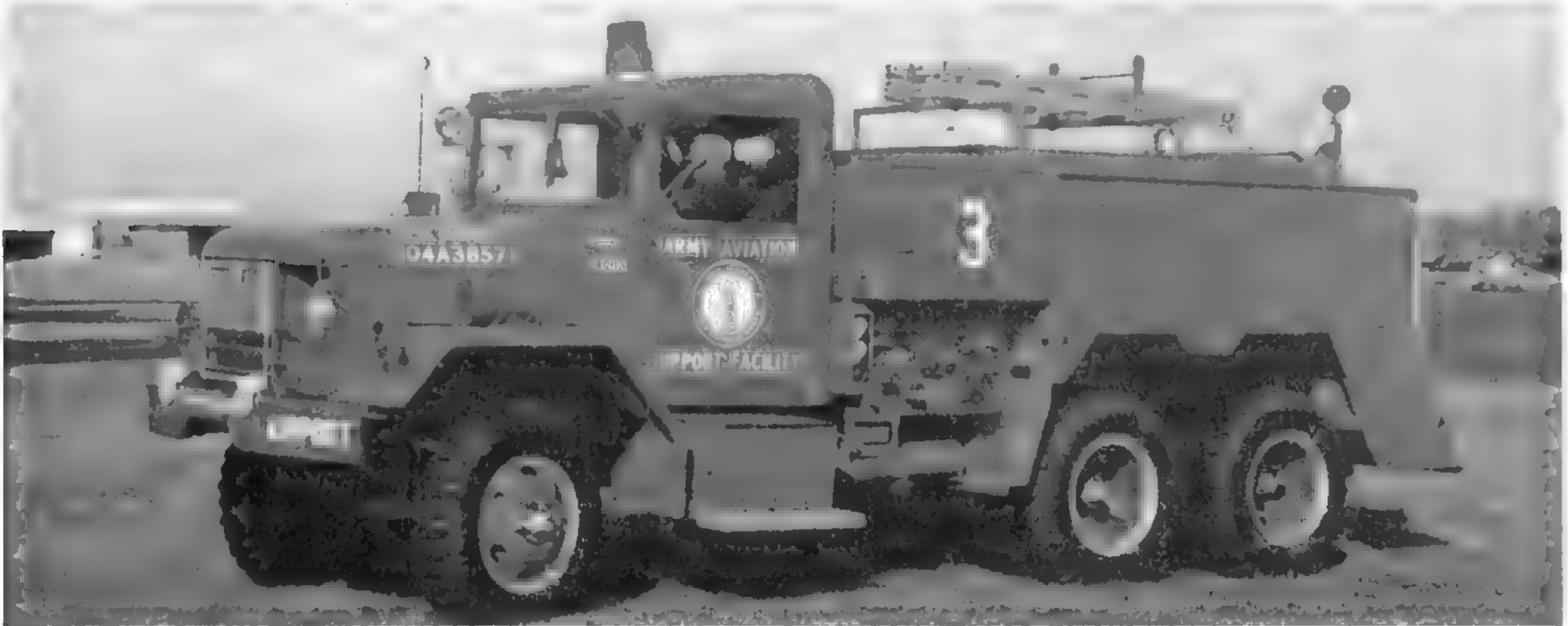
Later 530B trucks used dual 9.00 x 20 tires and multi-fuel engines, as shown in this example. Trucks in rear areas such as this one were initially painted a traditional red. This was later changed to a safety yellow paint scheme. (Photo courtesy of Richard Adelman collection)
